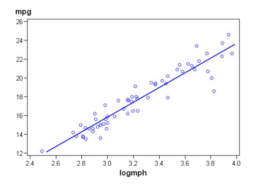
In the preceding example, the *t*-statistics came about by dividing the coefficient estimates  $b_0 = -7.796$  and  $b_1 = 7.874$  by their respective standard errors  $SE_{b_0} = 1.155$  and  $SE_{b_1} = 0.354$ .
